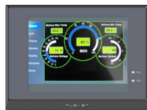
LCD-Touch screens, BMS/BMU controllers
